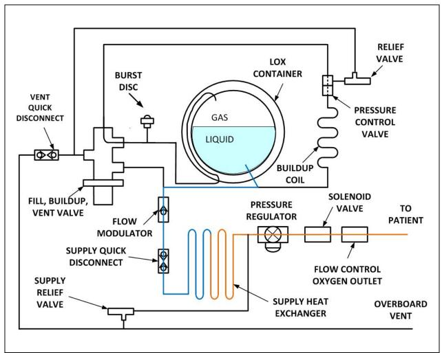
Figure 15 – Operating Mode Schematic
