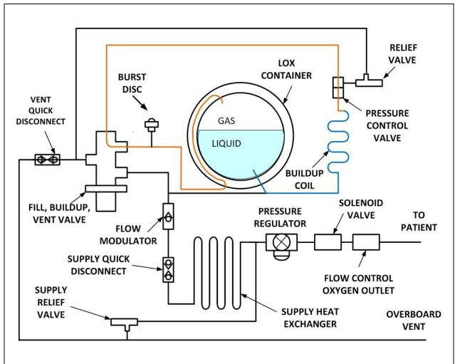
Figure 14 – Pressure Buildup Mode Schematic
