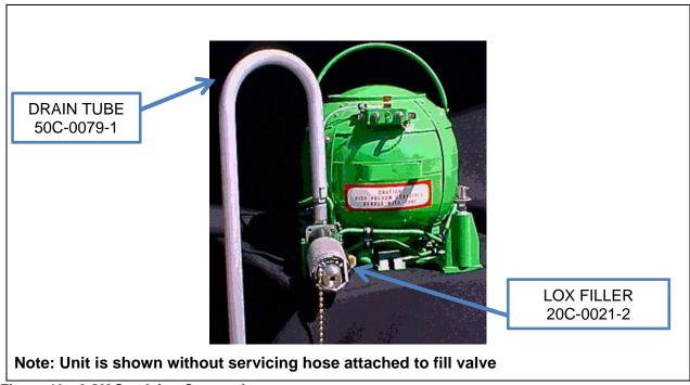
Figure 18 – LOX Servicing Connections
