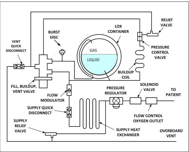
Figure 12 – LOX System Schematic
