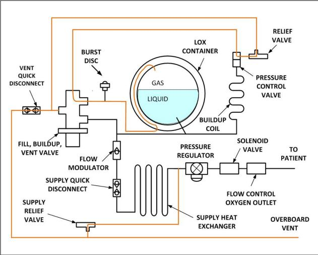
Figure 16 – Pressure Relief Mode Schematic
