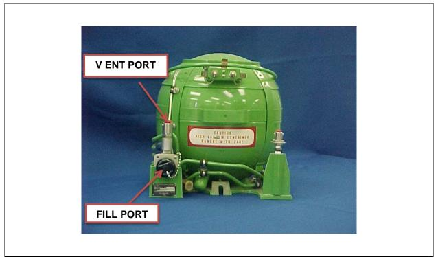
Figure 17 – Fill and Vent Port Locations
