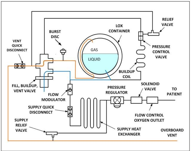
Figure 13 – Fill Mode Schematic
