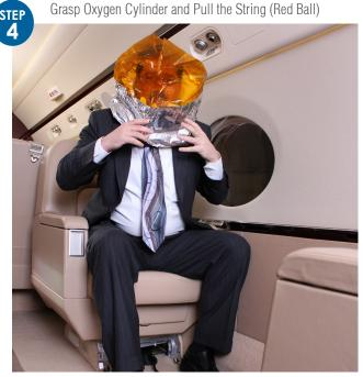
WARNING: Remove the hood immediately if the hood fails to slowly inflate after donning or if it collapses up against the face.
