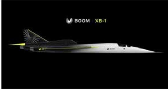
The purpose of the XB-1 is to be the one-third scale demonstrator airplane for Overture and being a critical step toward commercial supersonic travel.
